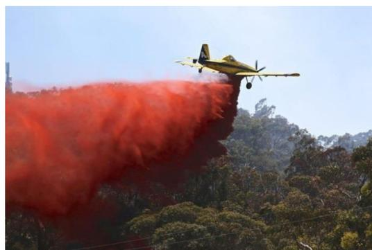
An 802 'Air Tractor' (SEAT) releasing a load of Phos-Chek fire retardant on vegetation
