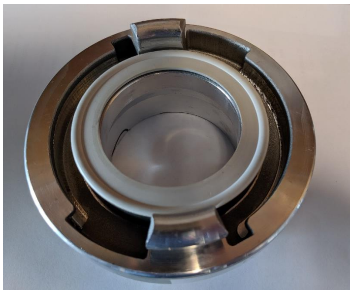
Photo 2 - Storz coupling showing a ribbed nitrile rubber sealing ring suitable for suction
