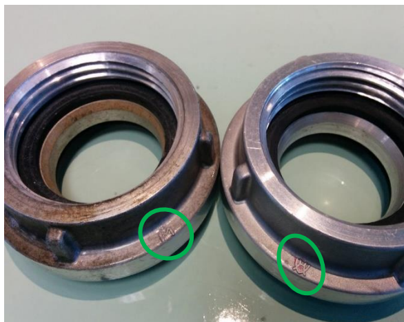
The above marks show the manufacturers mark and the forge mark.
